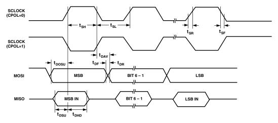
Figure 57. SPI Master Mode Timing (CPHA = 0)
